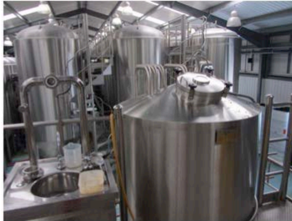
Front: processing hops. Back: the fermentation tanks
